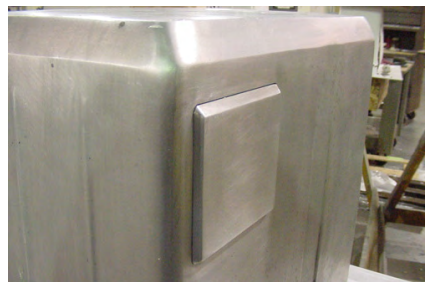
FIG. 10 Core pull tooling feature to assist in mold separation for formed parts with undercuts
